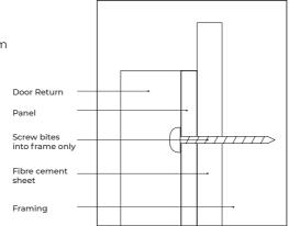
When fitting into an internal corner the first sheet will butt into the wall and allow for 3mm expansion while the second sheet will butt on to the first sheet allowing for expansion and contraction against the first sheet which was installed.
