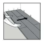
**9.** After 2-3 rows, adjust if needs be the distance between the front wall or skirting and the flooring edge and ensure adequate numbers of **6mm spacers** are in place to keep the flooring edge a minimum 6mm away from the wall or skirting at all points along this edge.
