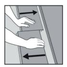
Secondly, **slide the short joints** of the board to be removed **horizontally in opposite directions**. **DO NOT** lift the end of a board to separate it as this will damage the end joint.
