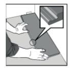
1. First board, first row. Place 6mm expansion gap spacers against the walls or skirting boards at the left hand end, and back long edge, of the first board and position the board end against the wall. The tongue on the back edge of the board should be against the spacers on the facing wall.
