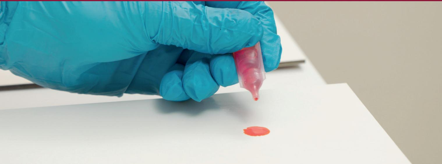
The hard, non-porous surface of the HPL and Compact ranges lends them very good stain and chemical resistance properties (as per EN438). The DURCON® Chemical compact range is more resistant to chemical products and detergents. Because the melamine-faced board is pressed at low pressure, it has lower resistance properties.
